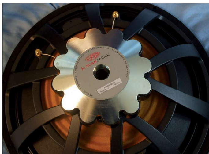
Photo 3: The 38WE frame is a really nicely configured 10-spoke (five double spokes) cast-aluminum frame with narrow 15mm to 25mm wide spokes to minimize reflections back into the cone.
